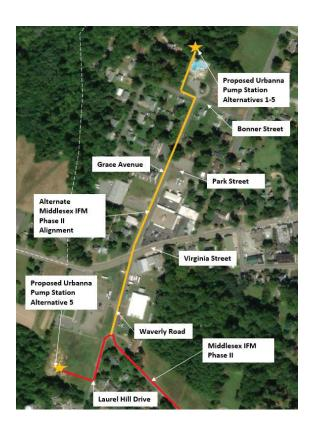
Figure 4-3: Urbanna Pump Station & Force Main Alignment Alternatives
