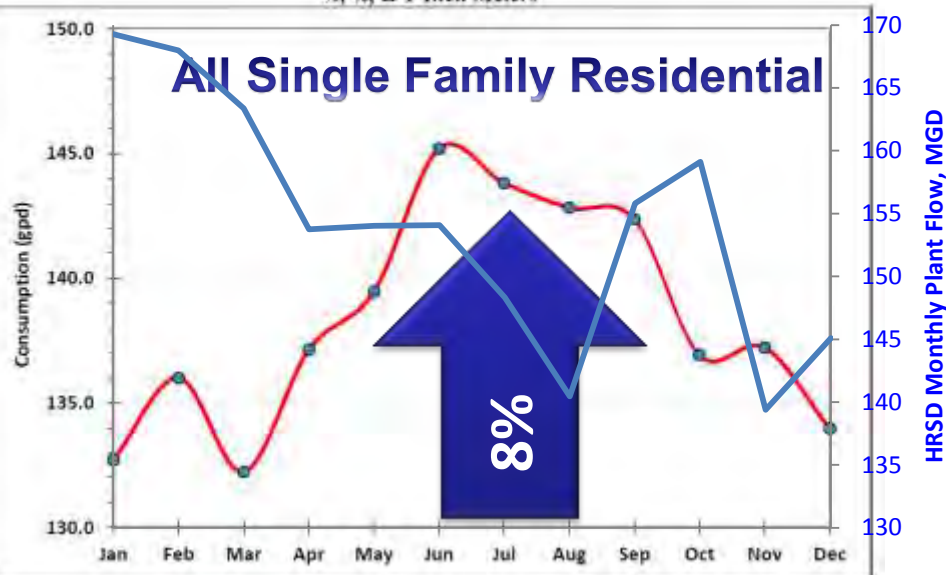
Figure 1 – Median Daily Monthly Consumption for All Single-Family Customers Consuming \geq 3 CCF per Month %, \frac{1}{2} , & 1-Inch Meters
