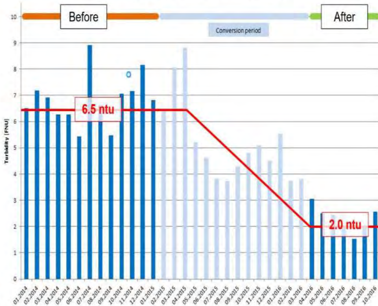
Turbidity in WWTP Effluent (Monthly Means)
