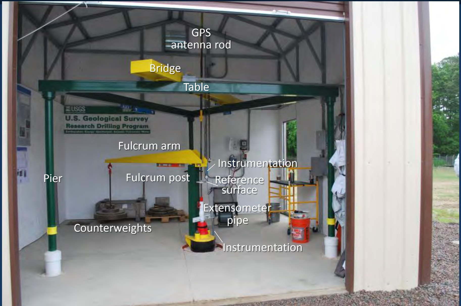
Extensometer layout
