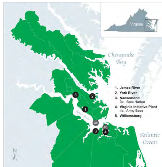
Figure 1. HRSD's service area, showing the locations of wastewater treatment plants with planned SWIFT facilities (1–5), with planned conveyance of service flows to a nearby plant with a planned SWIFT facility (3b), and with planned conveyance of secondary treated effluent to a nearby SWIFT facility (4b).
