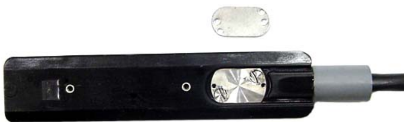
Figure 5-5 Low Profile Probe With Transducer Housing Revealed
