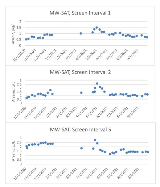
Figures 7, 8 and 9: Arsenic concentration in MW-SAT Screen 1, 2 and 5, respectively, values are in  $\mu g/L$ .
