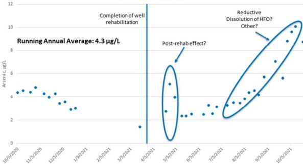
Figure 6: Arsenic concentration in MW-SAT Screen 9, values are in ug/L.
