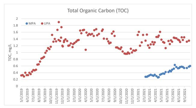
Figure 5: TOC concentration in the Upper and Middle Potomac conventional monitoring wells, MW-UPA and MW-MPA. Open symbols denote values < the detection limit of 0.2 mg/L.
