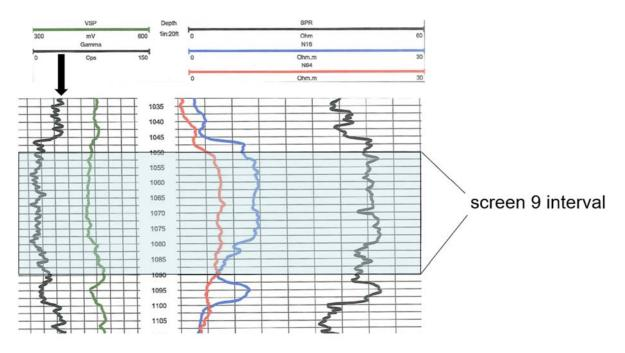
Figure 7: TW-1 geophysical log, gamma signal on the far left
