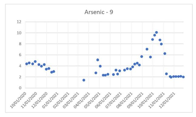
Figure 6: Arsenic concentration in MW-SAT Screen 9, values are in ug/L.
