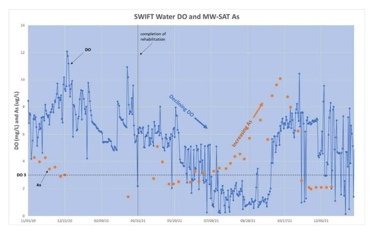
Figure 8: SWIFT Water Dissolved Oxygen and MW-SAT As concentrations
