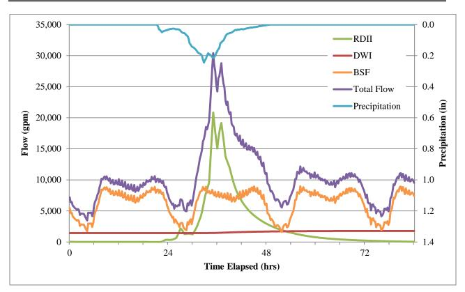
Figure 3-1. Example Components of Sewer Flow
