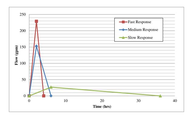
Figure 4-2. Synthetic Unit Hydrographs
