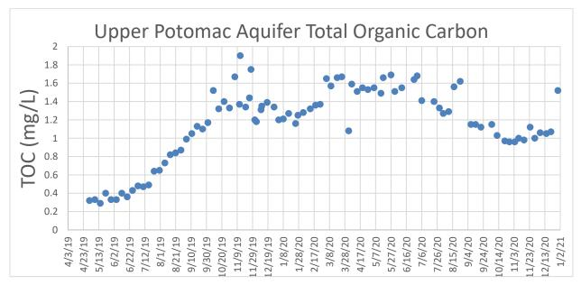
Figure 5: TOC concentration in the Upper Potomac conventional monitoring well, MW-UPA. TOC concentration in the October - November 2020 monitoring period in MW-UPA averaged 1.1 mg/L.
