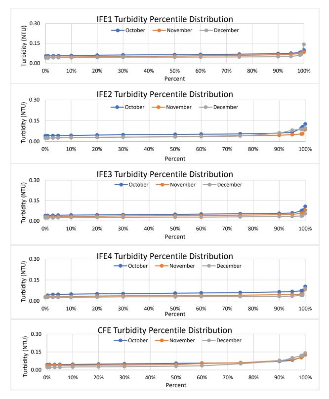
**Figure 1: Percentile distribution of 15-minute average Individual Filter Effluent (IFE) Turbidities for Biofilters 1-4 (IFE1-4) and Biofilter Combined Filter Effluent (CFE).** There were no 15-minute periods in this quarter with biofilter effluent turbidity values greater than 0.3 NTU. The 95% measured value for each biofilter IFE and the CFE was less than 0.15 NTU for each month in this quarter.
