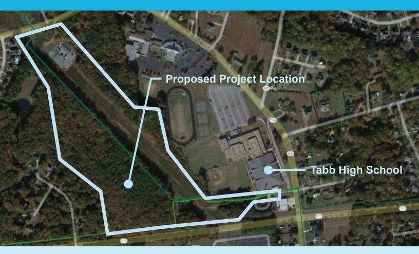
HRSD is looking to engage well-qualified partners to deliver a pressure reducing station and offline storage facility in Yorktown, Virginia. The project will include a 70'x130' pressure reducing station, 2.25MG Prestressed Concrete tank, utility work, and associated sitework. The current greenfield is located behind Tabb High School along Victory Boulevard.
