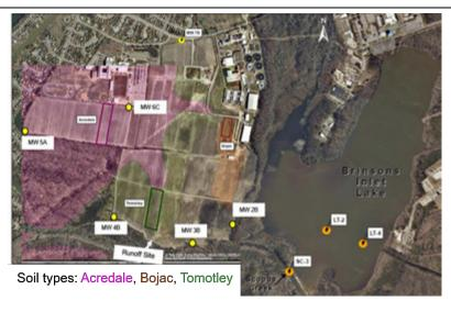
Figure 1. HRSD Progress Farm with monitoring wells, surface water sampling stations, and soil types.
