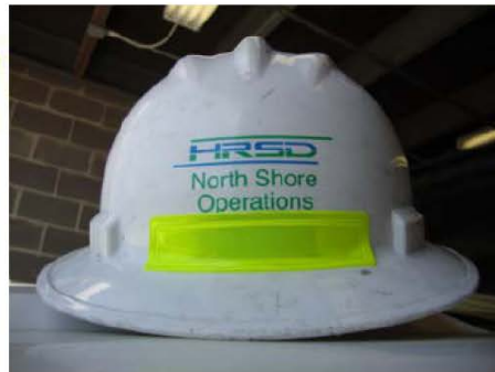
4"x1" retro-reflectivity strips on all four sides
