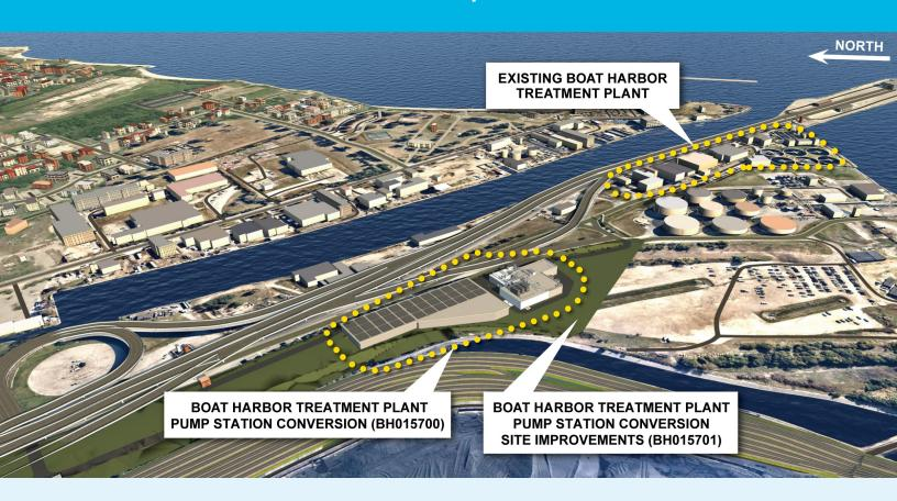
The Boat Harbor Treatment Plant in Newport News is closing to further reduce nutrient discharge to the James River Basin, supporting local water quality improvement and the Chesapeake Bay restoration effort. Construction of a new 36.5 MGD pump station will start soon to send the wastewater to HRSD's existing Nansemond Treatment Plant.
