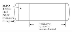
The diameter and sight glass measurements can be performed from the rear of the tank. If the highest sight glass is < 6" from the top, follow the drawing to the right.
