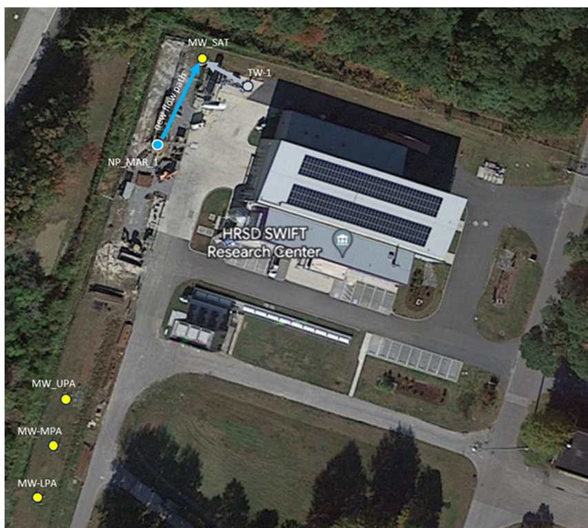
Figure 12, SWIFT Research Center Well Locations; Recharge water from NP_MAR_01 takes a different path to MW_SAT
